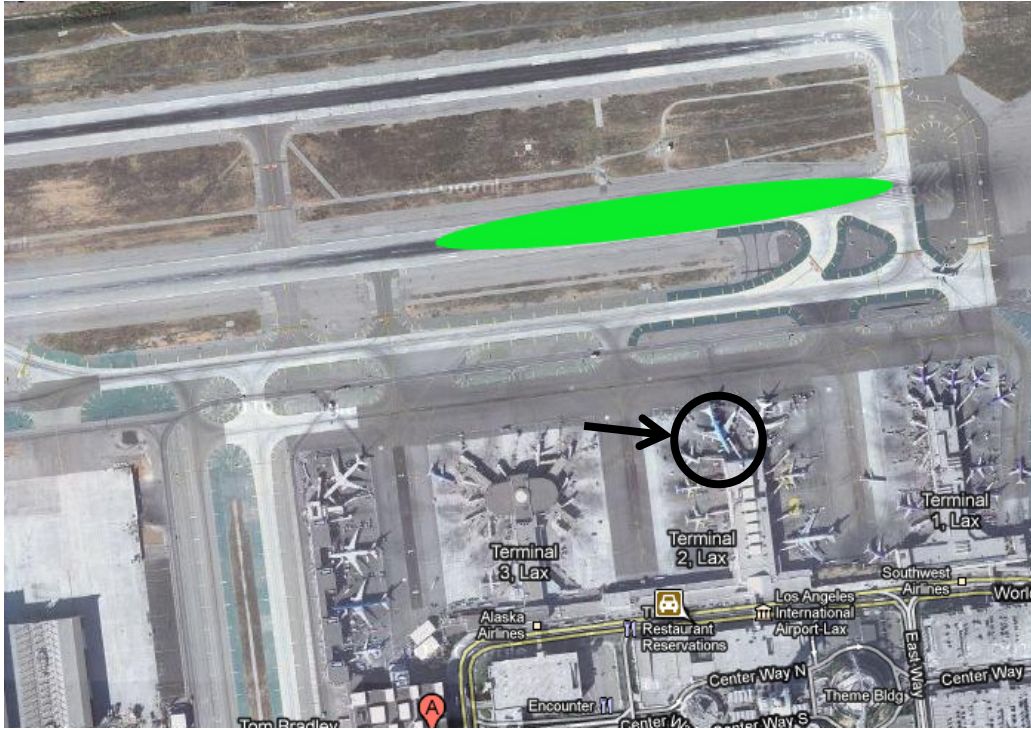
Figure 26. The airship's width and length are the main factor in determining airport compatibility. The airport shown is LAX, with scaled airship model and labeled 747.
